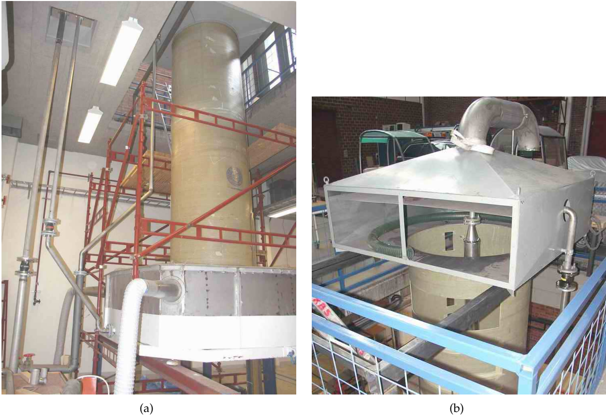
Figure 10.2: Rig Installation; (a) The Entrance Section and Tunnel, (b) Collector Hood.
