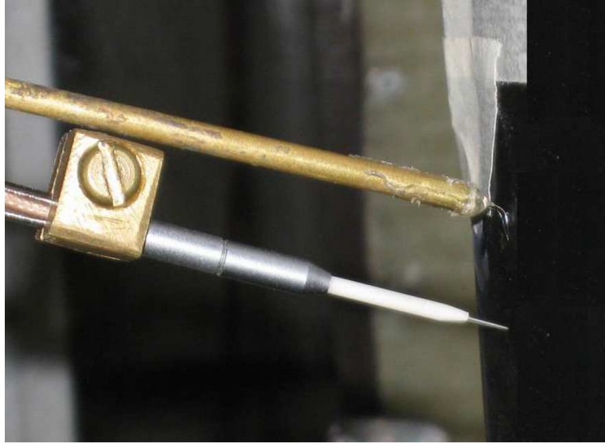
Figure 12.6: Thermocouple and cold-wire positions.
