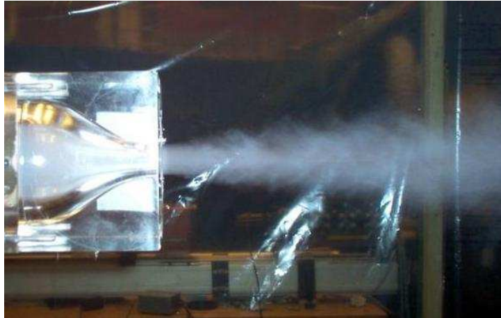
Figure 4.3: Smoke visualization of swirling jet used in experiments.
