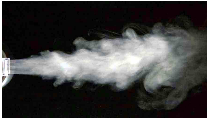
Figure 2.1: A jet flow visualization using a simple home humidifier.
