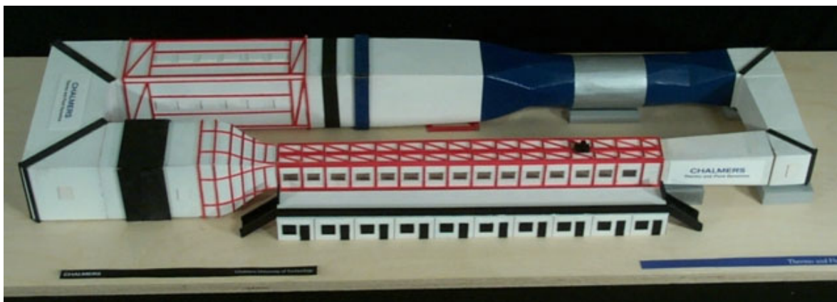
A 1:100 scale model of the planned Nordic Wind Tunnel.
