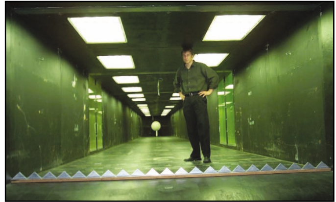
Example 1: BLWT 2, University of Western Ontario: Good overall size, insufficient flow quality (designed as wind engineering facility).
